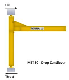
The diagram above details the thrust and pull forces that the jib crane applies to the supporting structure when a load is lifted. It is essential that a structurally adequate wall or column exists to support the jib crane. Contact your local Gorbel® dealer for specific thrust and pull forces.
