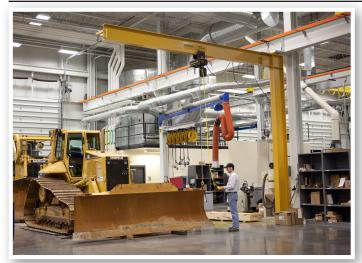
The MT Series Crane is floor supported, top stabilized, and is capable of 360° rotation via a top and bottom bearing assembly.
